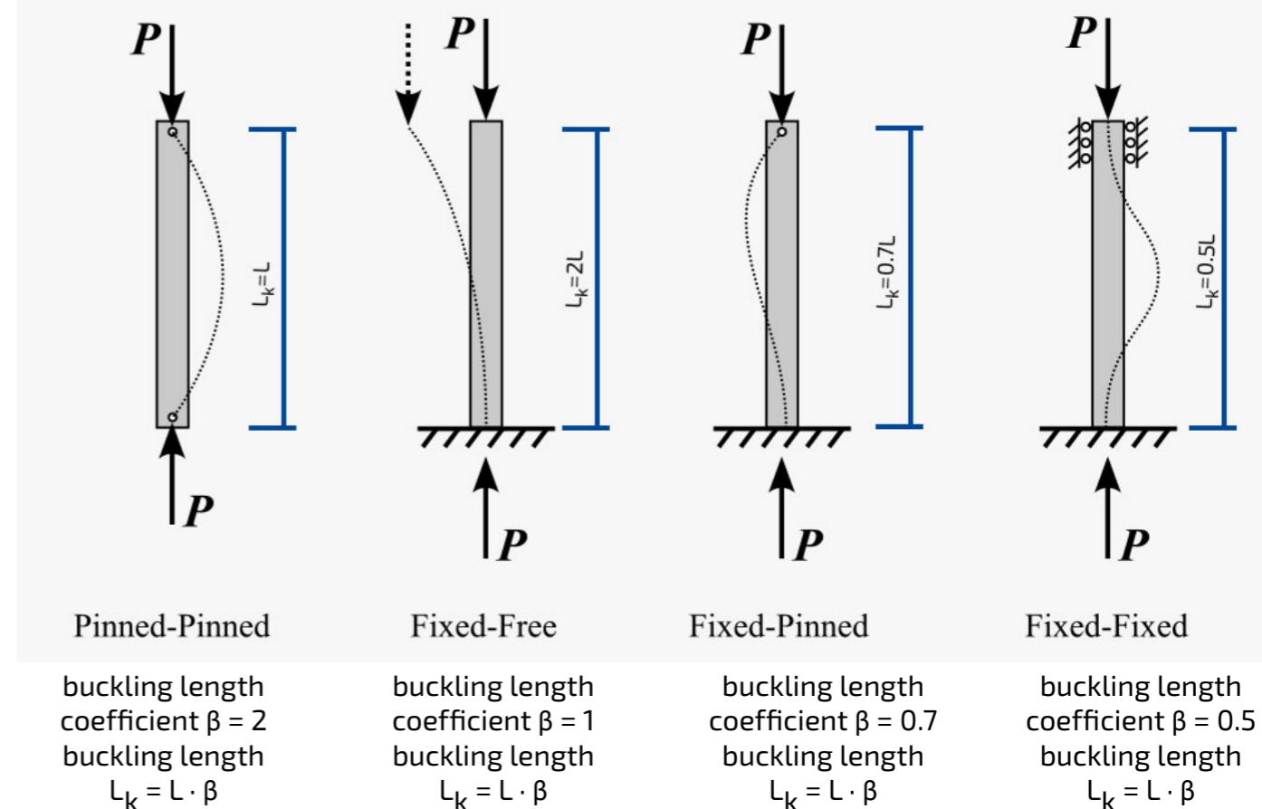
$P$  force,  $L$  bar length,  $L_K$  buckling length,  $\beta$  buckling length coefficient
